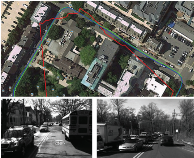
Fig. 9: (top) Ground truth (green), non-differential GPS (red), and GPS-denied navigation with pre-mapped landmarks (blue). (bottom) Examples of camera frames perceived during navigation.
