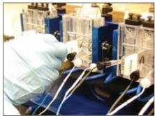
Figure 5: Top: Ussing absorption unit; Bottom: Slider with the intestinal tissues being mounted between the side-by-side compartmental unit of the Ussing system.
