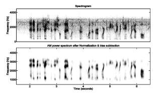
Fig. 3. Spectrogram of a renoised WSJ utterance corrupted with 15.6dB noise and Channel A characteristics (refer to Table 1) and it's normalized & bias subtracted amplitude modulation spectrum
