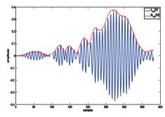
Fig. 1. A windowed narrow-band speech signal (in blue) and its corresponding AM signal (red) from the modified DESA algorithm.
