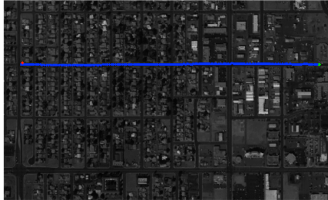
Figure 16. A straight but long track had high anomaly score because few tracks on this secondary street traveled that far before stopping or turning.
