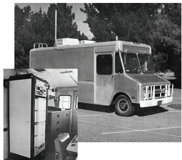
Figure 3-6. The SRI packet radio van. Inset shows two packet radios, an LSI-11 microcomputer containing TCP plus terminal interfaces, and a DataMedia terminal.
