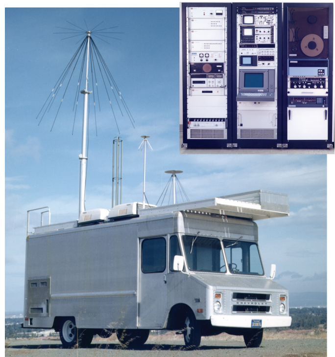
Figure 15-4. One of two radio spectrum monitoring vans built for the Iranian PT&T (November 1980).
