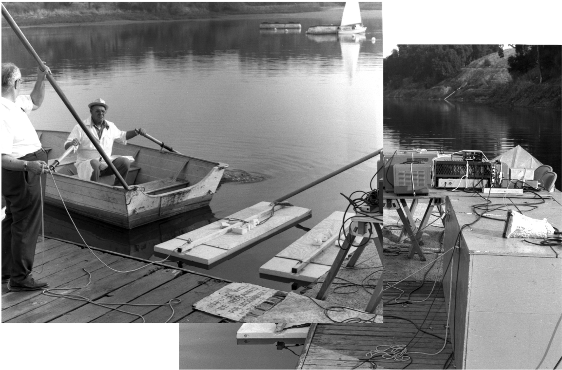
Figure 8-9. At Searsville Lake near Stanford University, location of SRI's active sonar experiments. Shown are acoustic equipment, hydrophones, with Jim Lomasney and Ernest Aho of the SRI "Navy"(about 1972).
