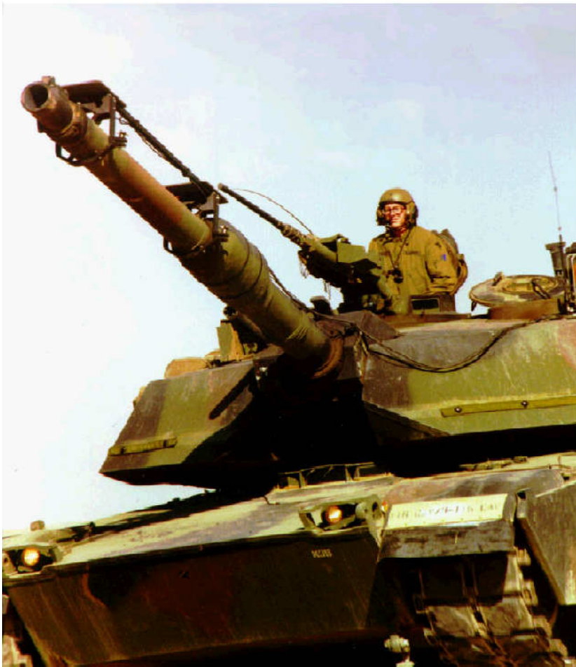
Figure 8-3. SRI's attitude-measuring jig mounted on the barrel of an Abrams tank.
