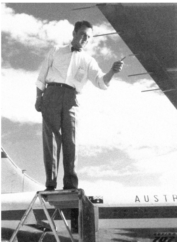
Figure 8-5. Some of the first SRI precipitation-static dischargers, their wing mounting location, and SRI's Dr. Joe Nanevicz.
