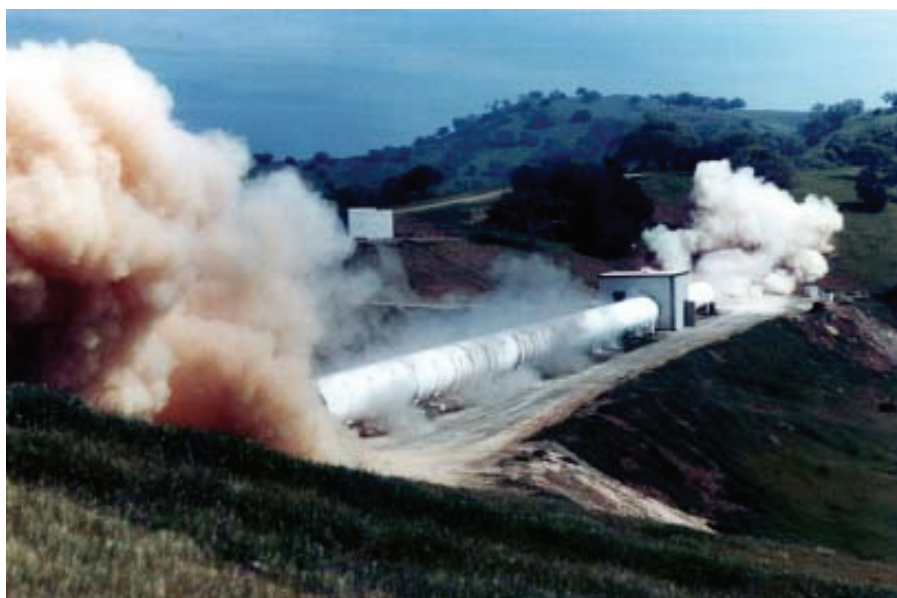
Figure 11-9. SRI's Corral Hollow test site near Livermore, CA, showing the eight-foot shock tube in use.
