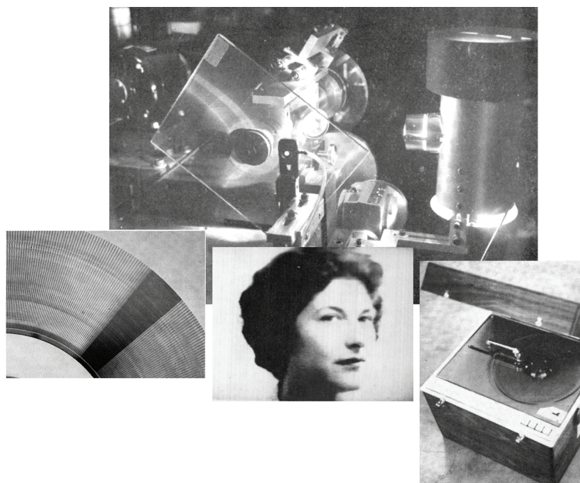
Figure 7-4. SRI optical recorder with insets showing an analog disc where each 180-degree annular trace created one frame, a reproduced image, and the final lab prototype of a playback unit.
