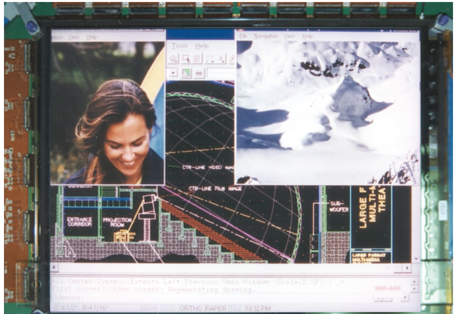
Figure 7-11. A prototype of a 14-inch field emission display made by Candescent of San Jose, CA (image received May 2000).
