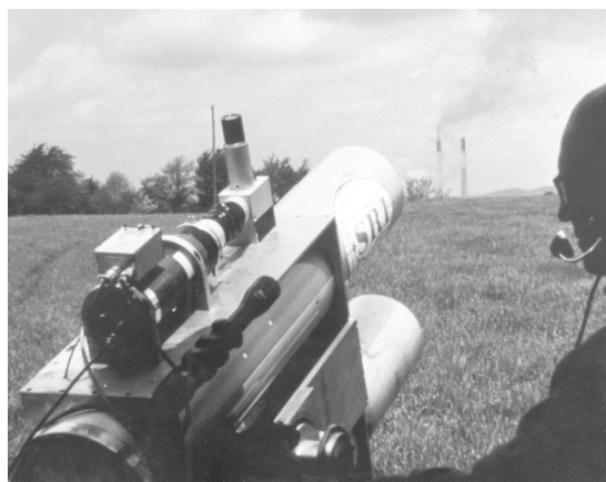
Figure 9-19. An SRI lidar in the field being used to detect effluents from smoke stacks in western Pennsylvania in 1968.
