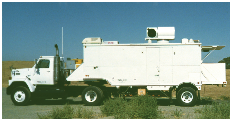
Figure 9-21. SRI lidar van used in the detection of trace levels of atmospherically transported chemical agents.
